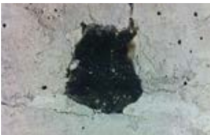
Close-up of a concrete cross-section showing the swelling properties of PENEBAR SW waterstop.
